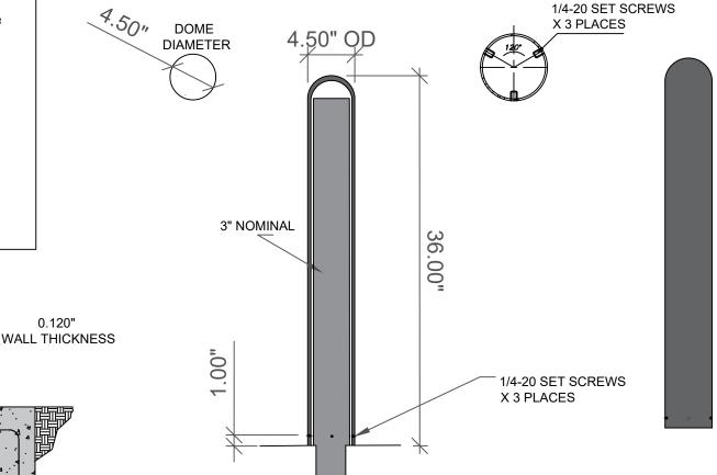
SPECIFICATIONS HEIGHT: 36" DIAMETER: 4.50" WALL THICKNESS: 0.120" DOME (SHOWN) STANDARD FLAT SLOPED REVEAL
